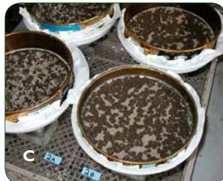
FIGURE 2.24 A-C. Aggregate Stability test. A rain simulator is used for 5 minutes on a sieve containing soil aggregates.
