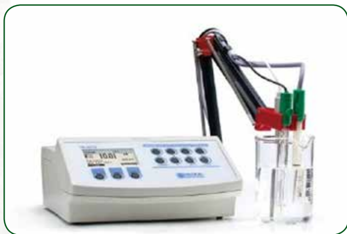
FIGURE 2.51. Electrical conductivity (EC) meter used to measure salinity.
