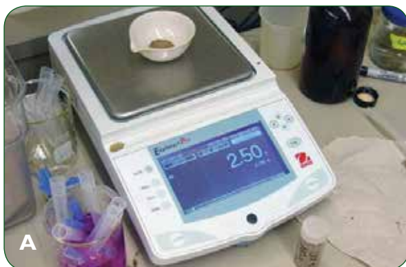
FIGURE 2.36 A and B. A 2.5g sample of soil is placed in a centrifuge tube filled with \text{KMnO}_4 solution (A). Absorbance is measured at 550 nm (B). The more active carbon found in the soil sample, the lighter the color of the solution.
