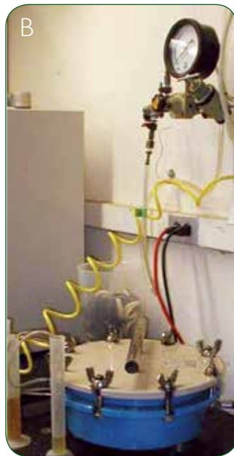
FIGURE 2.15 A-C Ceramic plates with soil (A) are inserted into high pressure chambers (B). Equilibrated samples at target pressure (C). Samples are weighed and then oven dried overnight.
