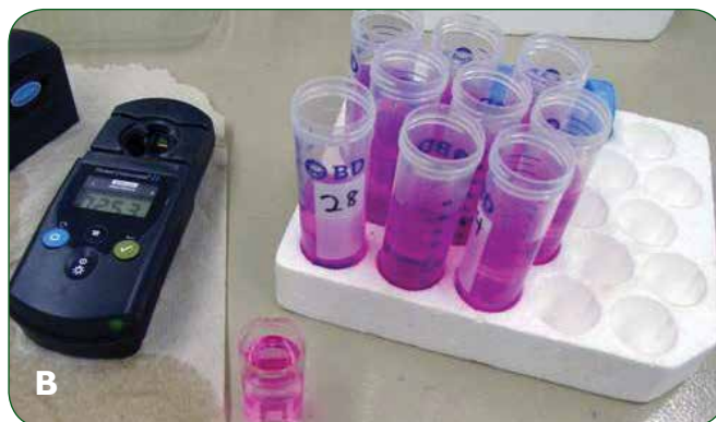
FIGURE 2.36 A and B. A 2.5g sample of soil is placed in a centrifuge tube filled with \text{KMnO}_4 solution (A). Absorbance is measured at 550 nm (B). The more active carbon found in the soil sample, the lighter the color of the solution.
